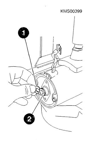
Checking and adjusting armature axial clearance
